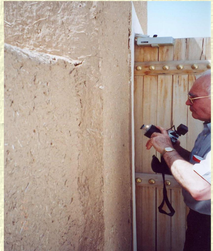
Magnified photographing of plaster using Dermaphot lens
